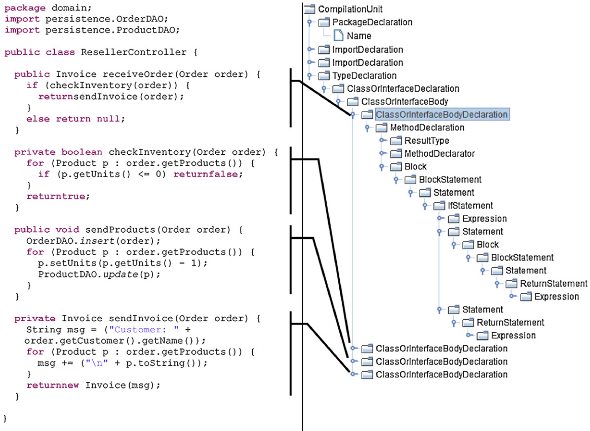
Fig. 1. An example of the L0-to-L1 transformation for a product shipping system.
