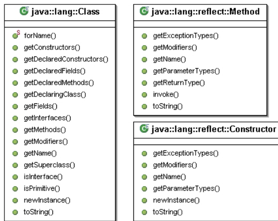
Figure 9. UML representation of the Class and Method Java classes.
