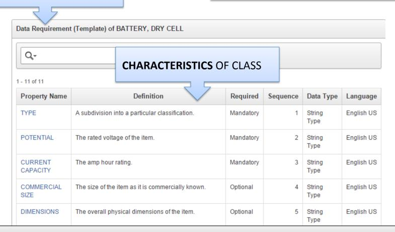
**Example** of Data Requirement to show *Class* **BATTERY, DRY CELL** and *Characteristic Data*
